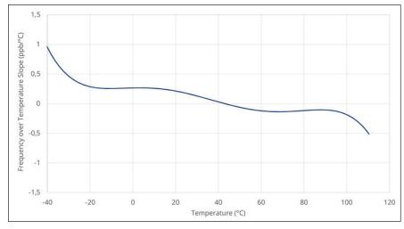
> The SiT5977 operates at ±1 ppb/°C stability over temperature slope (dF/dT) to ensure a precise time reference under thermal shock and airflow. This means no performance throttling, fewer dropped packets and smaller windows of uncertainty.
