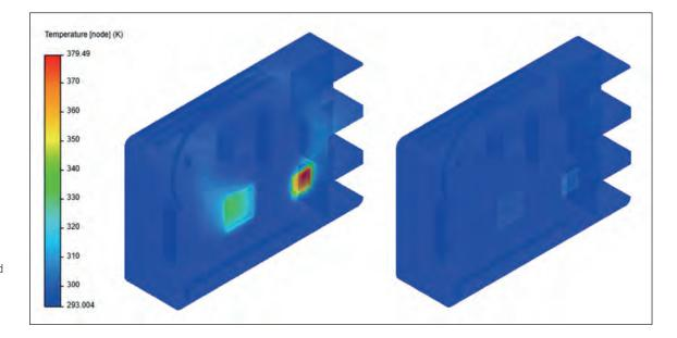
Thermal radiation comparison of the same heat-sink in air (on the left) and in Submer's SmartCoolant (on the left).
